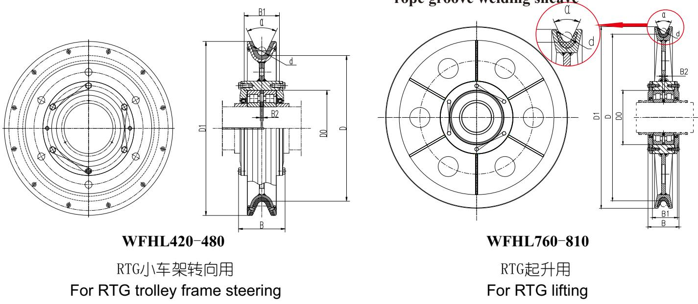
图7 复合绳槽焊接滑轮 Fig. 7 Composite rope groove welded sheave
