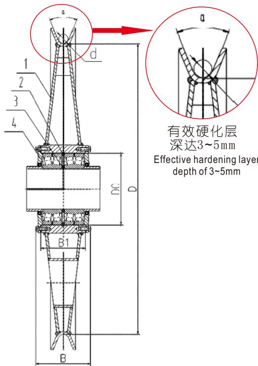
1-焊接滑轮 Weld sheave; 2-外隔圈 Outer spacer 3-内隔圈 Inner spacer; 4-端盖 End cover
