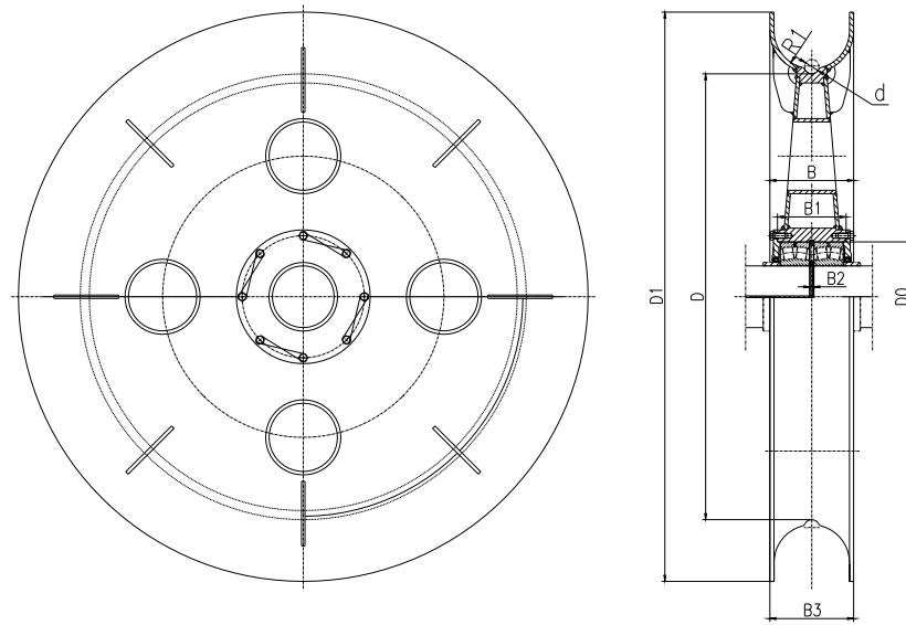
图6 宽槽焊接滑轮 Fig. 6 Wide groove welded sheave
